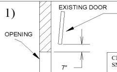
**1.1)** If you want the security door to come down parallel with opening then readjust existing door so that in the full up position the bottom will be a minimum of 7 inches above the top of the opening.
