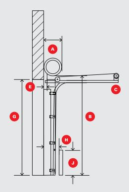
**NOTES:** A torsion bar support is required on all doors 10' or wider. The Rasco door has outside pull brackets / cables.
