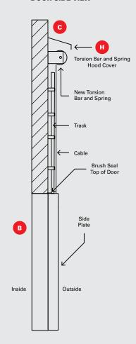
NOTES: A solid shaft is required on all doors 12' or wider or motorized.
