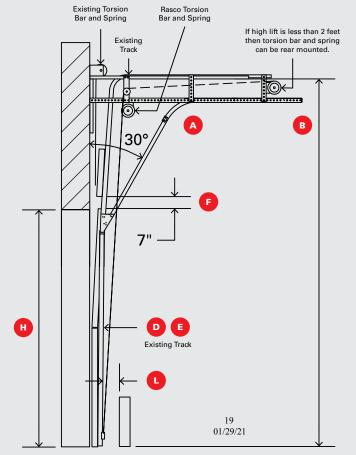
NOTES: A torsion bar support is required on all doors 10' or wider. Switch track cannot be used if existing door has outside pull cables or has TKO, Workhorse or Barcol type tracks. The Rasco door has outside pull brackets/cables.
