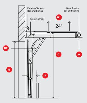
NOTES: A torsion bar support is required on all doors 10' or wider. Switch track cannot be used if existing door has outside pull cables or has TKO, Workhorse or Barcol type tracks. The Rasco door has outside pull brackets/cables.
