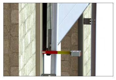
Distance from wall to furthest part of existing track at top of the opening
