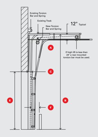
**NOTES:** A torsion bar support is required on all doors 10' or wider. Dual track cannot be used if existing door has outside pull cables.
