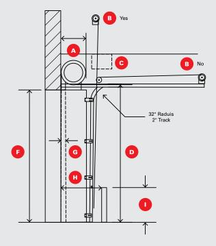
NOTES: A torsion bar support is required on all doors 10' or wider. The Rasco door has outside pull brackets/cables.
